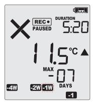
Tip: Pressing and holding the Tip: Pressing and holding the button will get you back to the previous screen, rather than advancing one screen.
