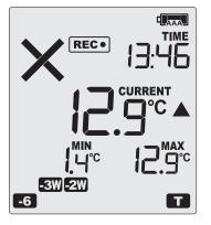
Each alarm trigger condition consists of a threshold temperature value, an activation type (which can be instant, consecutive or accumulative<sup>2</sup>) and a delay time, if it is not an instant alarm.
