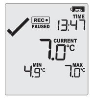
How long **PAUSED** is displayed depends on when between readings you press the button. It will show longer, if the button is pressed just after the logger takes a reading, but shorter if you press the button just before. For example, if you configure a logging interval of 10 minutes and 2 paused readings, the time **PAUSED** is shown could be as short as 10 minutes, but as long as 20 minutes.
