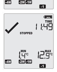
Once the logger has stopped, the last alarm status before the logger stopped will continue to be indicated with a cross or a tick symbol on the display, but the audible alarm and the alarm LED will turn off (see exception <u>below</u>).
