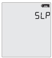
A hibernated logger cannot be reactivated via the buttons - it must be reconfigured with LogTag<sup>®</sup>. Analyzer.
